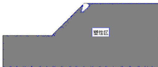
图7 \nu=0 时的塑性区分布 Fig. 7 Distribution of plastic zone with Poisson's ratio \nu=0
