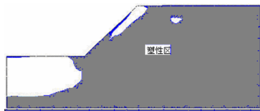
图8 \nu=0.3 时的塑性区分布 Fig. 8 Distribution of plastic zone with Poisson's ratio \nu=0.3
