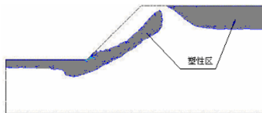
图9 \nu=0.49 时的塑性区分布 Fig. 9 Distribution of plastic zone with Poisson's ratio \nu=0.49
